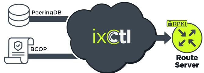
IXctl takes data directly from PeeringDB and combines it with industry best practices to generate (and maintain) secure route server configurations.
